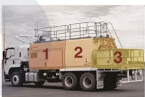
Segmented tank design
