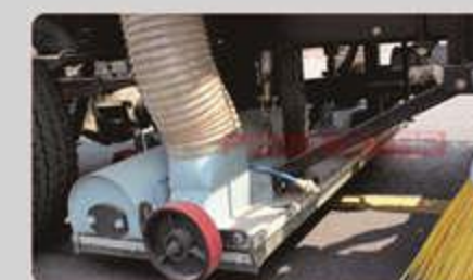
Patent design water spraying system for dedusting
