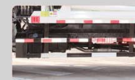
Safety fence at two sides
