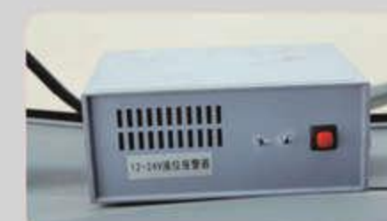
Level alarm system, in cabin
