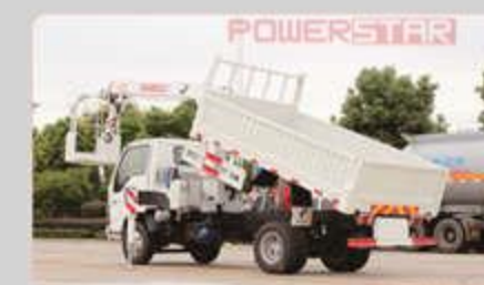
Tipper with work cage
